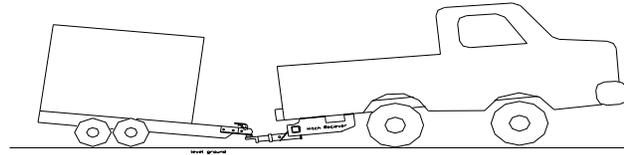
1) Line up the towing vehicle and trailer on level ground in the straight ahead position, uncoupled.
