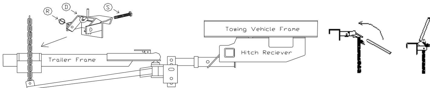
**Warning:** If the chain is angled while in the engaged position on the clamp, it may cause binding or buckling while turning, causing damage to the clamps or bars. This will void the warranty of the weight distribution system!
