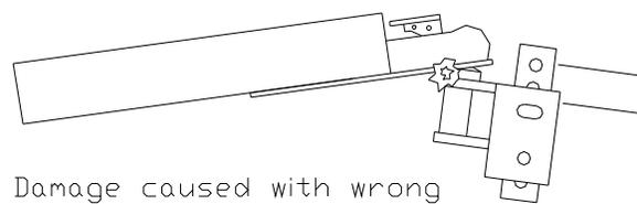
Damage caused with wrong hitchball will not be covered under warranty
